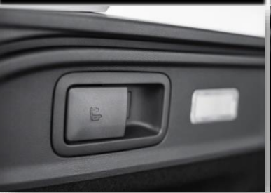
'Magic Flat' rear seat release switch
